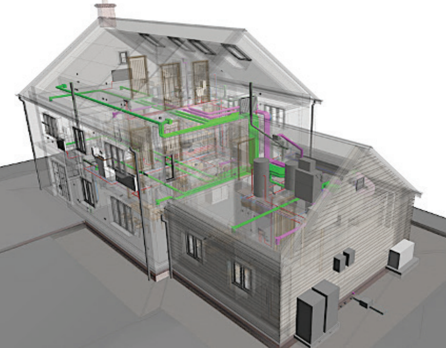
Figure 2: Revit model showing MVHR layout
